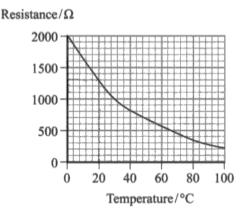
(i) Use the graph to find the resistance of the thermistor at 20 °C.
